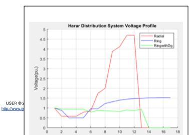
As it can be observed the ring voltage profile of all buses except bus 1 is below the minimum threshold value
