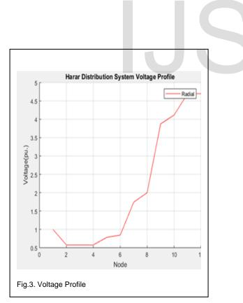
Fig.3. voltage profile for radial Harar distribution system. As it can be observed the radial voltage profile of all buses except bus 1 are below the minimum threshold value (0.95pu) and Bus 6,7,8,9,10,11,12 are above a maximum
